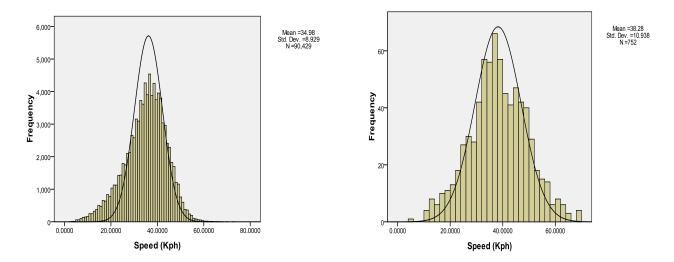
Examination of the distributions establishes that around a quarter of the combined group of scooter and motorcycles (502 of 1892 observations) were travelling at a speed equal or greater than the 85% percentile speed of car traffic.
